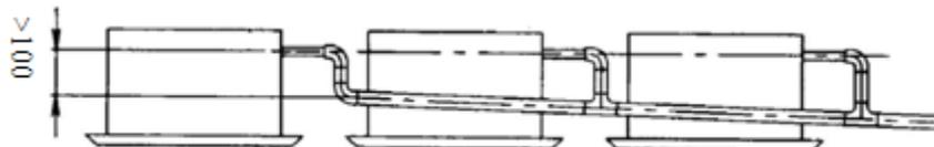
After installation, conduct drainage test to determine if water correctly flows through pipeline and carefully observe the connection to ensure there is no leakage. If the unit is installed in new house, it's recommended to test before decorating ceiling. Conduct drainage test for the unit used for heating only.
