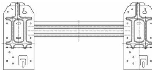
The wall for installing indoor unit should be firm to prevent vibration. Horizontally install hanging plate on the wall with four cruciform screws to keep laterally horizontal and longitudinally vertical.
