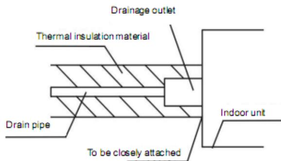
Thermal insulation material should be rubber & plastic thermal insulation pipe with thickness above 10mm
