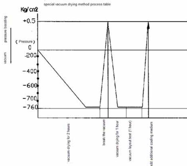
Method is that insert break the nitrogen vacuum work procedure for more than one time during common vacuum drying process.
