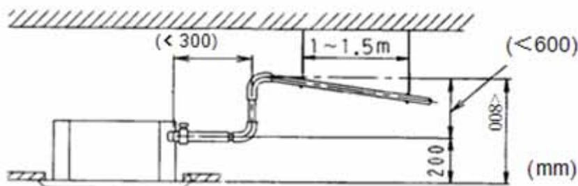
When install drain pipes for multiple units, it's necessary to install utility piping at 100mm under the drainage outlet of each unit as shown in the following diagram.
