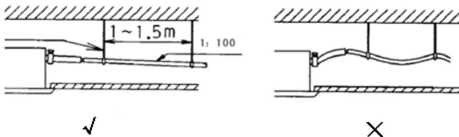
Although draining pump of unit has a lift of 1200mm, considering the protective shutdown of float switch will be caused due to the back flow of condensed water after shutdown, please arrange drain pipe according to the following diagram where possible.
