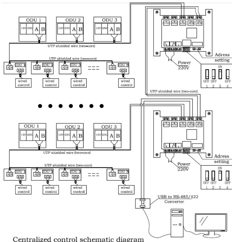
Centralized control schematic diagram
