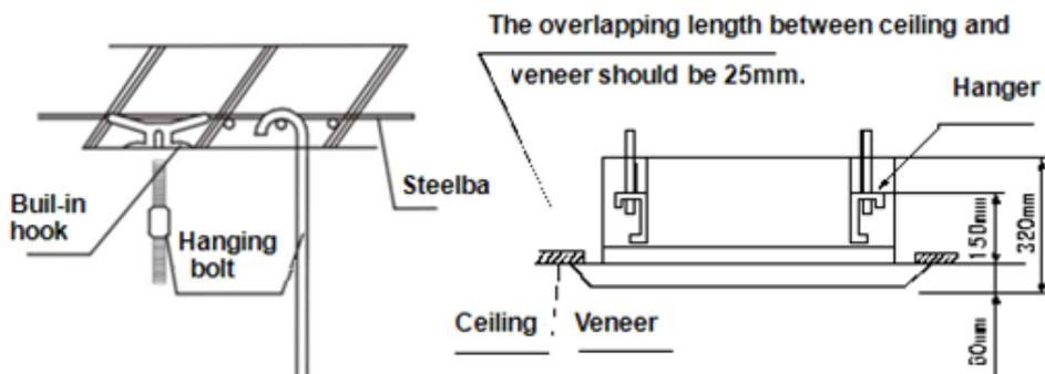
If the unit body is installed on oblique ceiling, it’s necessary to put cushion block between ceiling and air outlet panel to ensure the unit body is installed on horizontal position.
