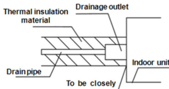
Thermal insulation material should be rubber & plastic thermal insulation pipe with thickness above 8mm.
