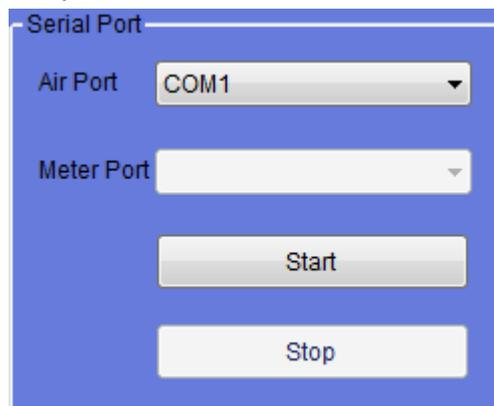
In the interface, Air Port is the communication port with ARV system. If there is more than one port selection in the drop down box, then customer must choose the port generated from USB-485 transformer.
