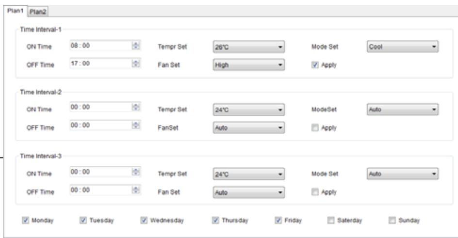
temperature as 26°C and turn off units at 17:00 p.m. from Monday to Friday, and turn on units at 9:00 a.m. in cooling mode with a setting temperature as 26°C and turn off units at 15:00 p.m. on Saturday and Sunday, then the pan is set as below:
