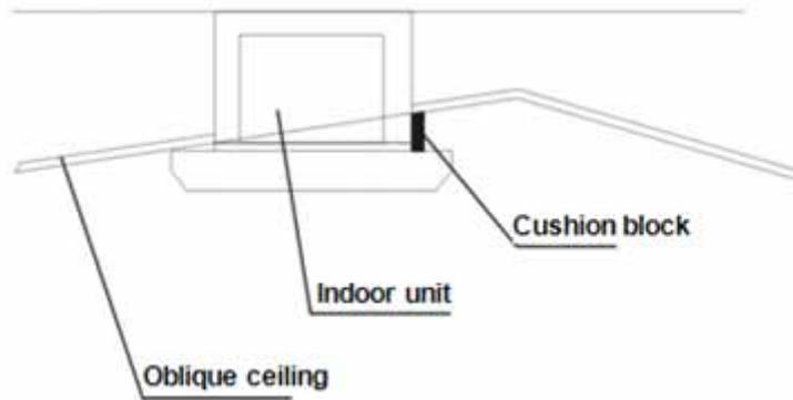
Dual nuts should be adopted to fix the indoor unit under the ceiling.
