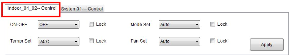
2) Control ports in IDU interface can realize functions such as on/off、 mode selection、 temperature control、 wind speed selection etc.. Besides, Lock function can realize locking of the above four functions. Remote-controller and wired controller can't control IDUs after locking. Click “Apply” button to send command after finishing the above operations.
