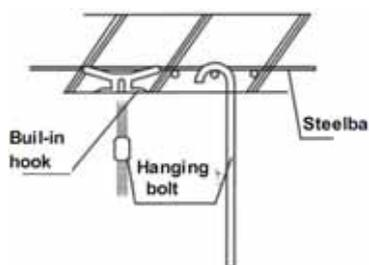
Fixing of hanging foundation: Fix hanging bolt as shown in the diagram or fix it with iron bracket and wooden bracket.
