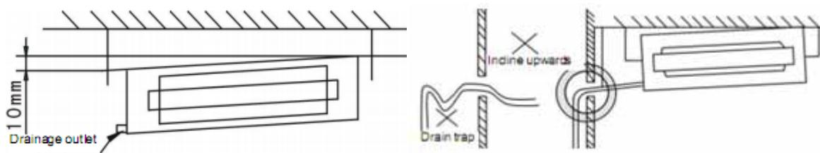
After installation, conduct drainage test to determine if water correctly flows through pipeline and carefully observe the connection to ensure there is no leakage. If the unit is installed in new house, it's recommended to test before decorating ceiling. Conduct drainage test for the unit used for heating only.
