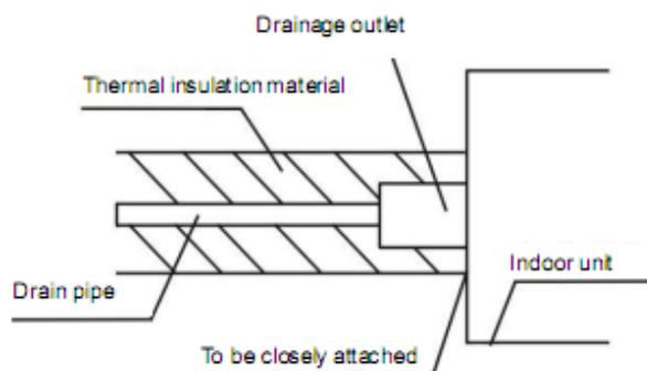
Drain pipe should incline downwards with gradient of 1/50-1/100, which will subject to failure such as back flow or water leakage in case of up-and-down fluctuation or upward inclination.
