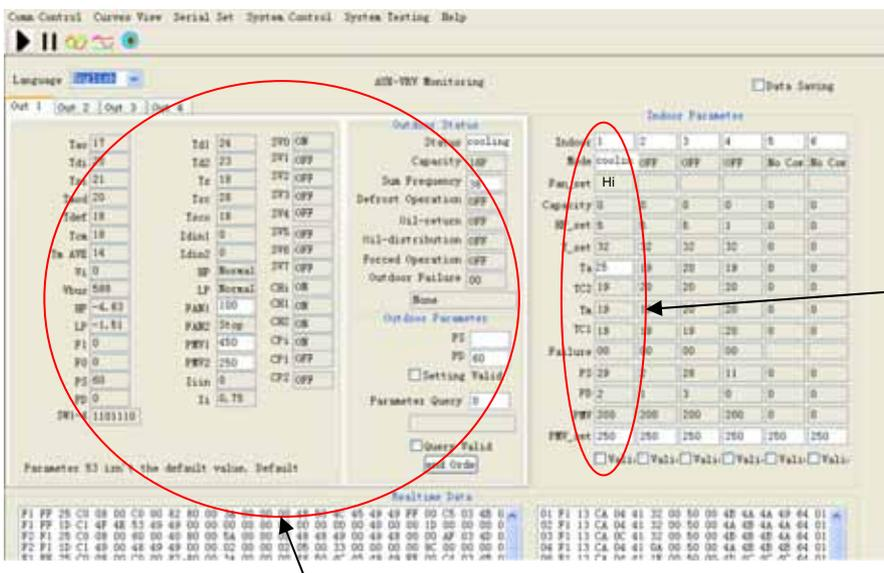
Open cooling mode of No. 1 indoor unit and observe the state:
