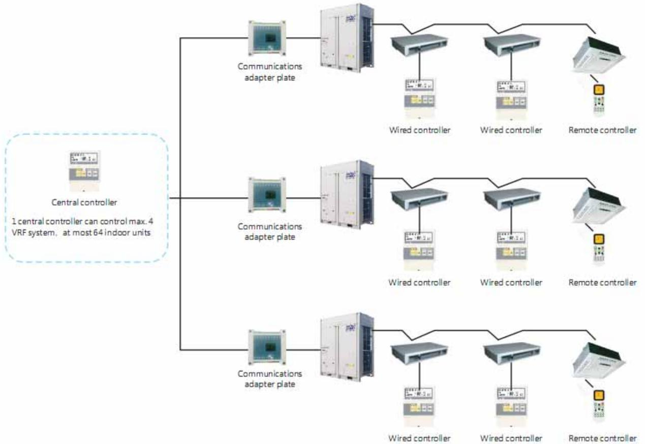
**Wiring Diagram among Adapter Plate, Centralized Controller, Weekly Timer and Monitor**
