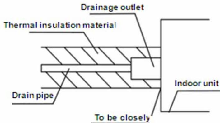
Thermal insulation material should be rubber & plastic thermal insulation pipe with thickness above 8mm. Drain pipe should incline downwards with gradient of 1/50-1/100, which will subject to failure such as back flow or water leakage in case of up-and-down fluctuation or upward inclination.
