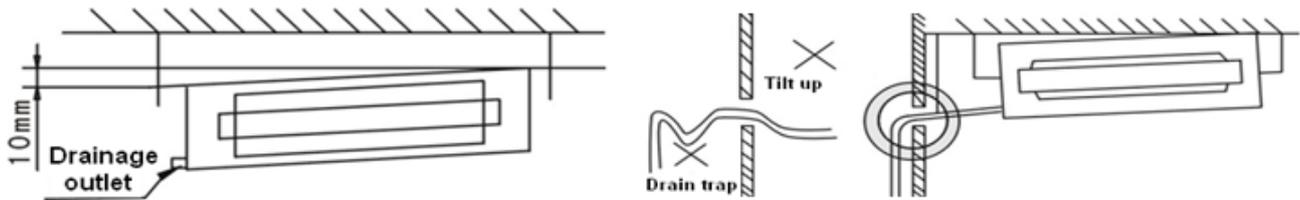
When finish installation please carry out the drainage test to ensure that the water flow through the pipeline fluently, and carefully observe the junction to ensure that there is no water leakage at the junction. If the unit is installed in the newly built house, strongly recommend that this test taken before the ceiling installation. Even it is the heating only unit, this test is unavoidable.
